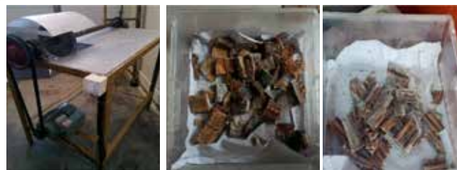
Semi- automatic dryfish cutter
