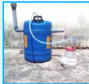
Laboratory scale biogas production unit
