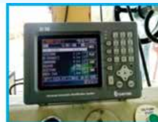
Fishing vessel fitted with Universal Automatic Position Identification System
